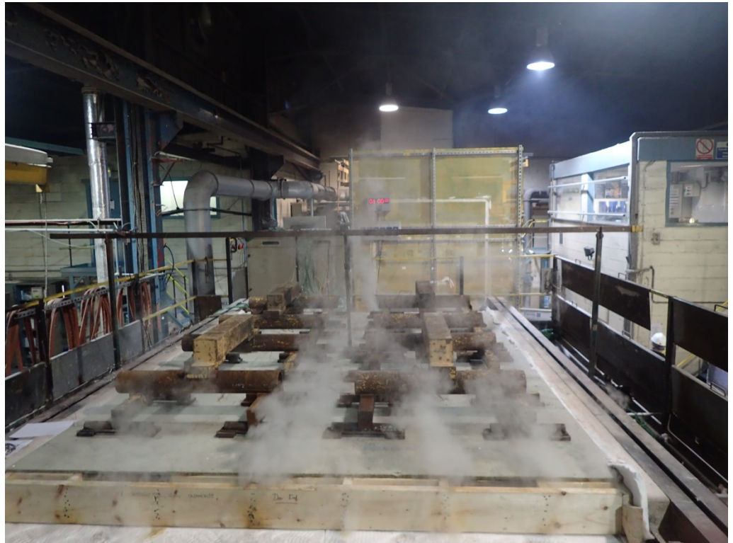
The unexposed face of the assembly after a test duration of approximately 60 minutes
