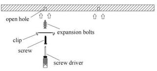
C. Open the end with input mask according picture 1 & picture 2,then open corresponding preset line hole according to th input cord loaction, pictures 3, and fix the cord clip.
