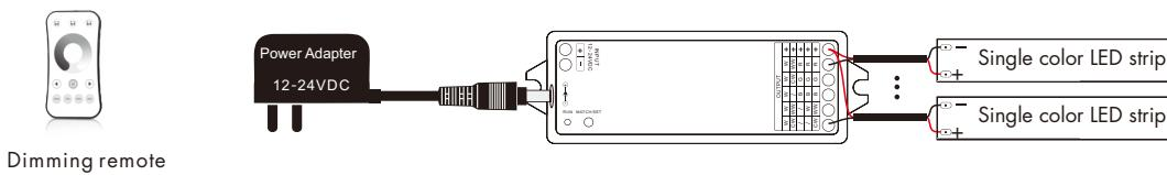
Press and hold match/set key for 8s, until the RUN LED indicator turn white, then release, the controller will become DIM type, then do smart config by Tuya smart APP, or short press match key to match with dimming RF remote.
