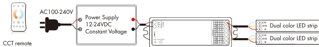
Press and hold match/set key for 10s, until the RUN LED indicator turn yellow, then release, the controller will become CCT type, then do smart config by Tuya smart APP, or short press match key to match with CCT RF remote.
