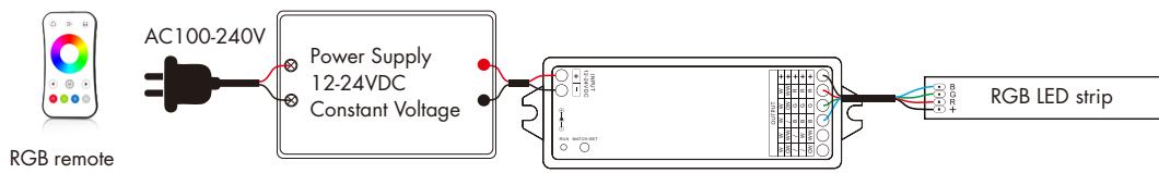
Press and hold match/set key for 12s, until the RUN LED indicator turn red, then release, the controller will become RGB type, then do smart config by Tuya smart APP, or short press match key to match with RGB RF remote.
