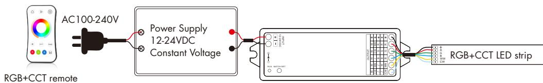
Press and hold match/set key for 16s, until the RUN LED indicator turn blue, then release, the controller will become RGB+CCT type, then do smart config by Tuya smart APP, or short press match key to match with RGB+CCT RF remote.
