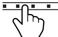
1.2 Stick the strip and carefully press down on the strip for about 10secs (avoid pressing on the LEDs).
