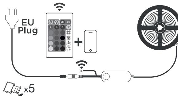
Connect the power supply, controller, and light strip. Then connect it to the AC power grid.
