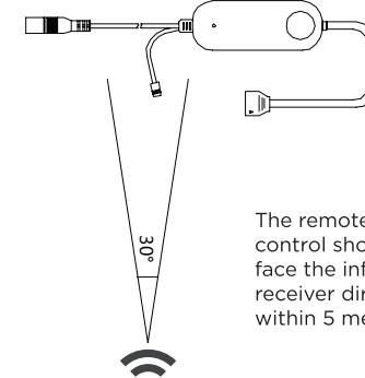
The remote control should face the infrared receiver directly, within 5 metres.
