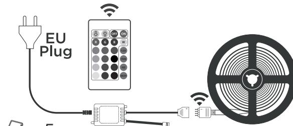
Connect the power supply, controller, and light strip. Then connect it to the AC power grid.
